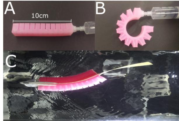
Fig. 1. A) An uninflated pneunet connected to a syringe. B) A fully inflated pneunet. C) As seen from below, a pneufish operating in water. The cuff (left end of the pneufish) connects to a dorsally-located vertical rod housing the force and torque transducer. Image C adapted from [8].
